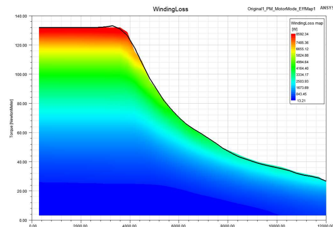
仅考虑绕组直流损耗 ( R_{dc} = 0.015 \Omega )
